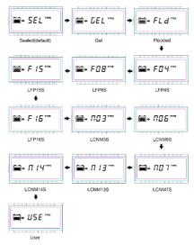
Note: If the controller supports 48V system voltage, the battery type will display LiFePO4 F15/F16, and Li(NiCoMn)O2 N13/N14.
