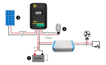
Figure 2-2 Schematic of wiring diagram
